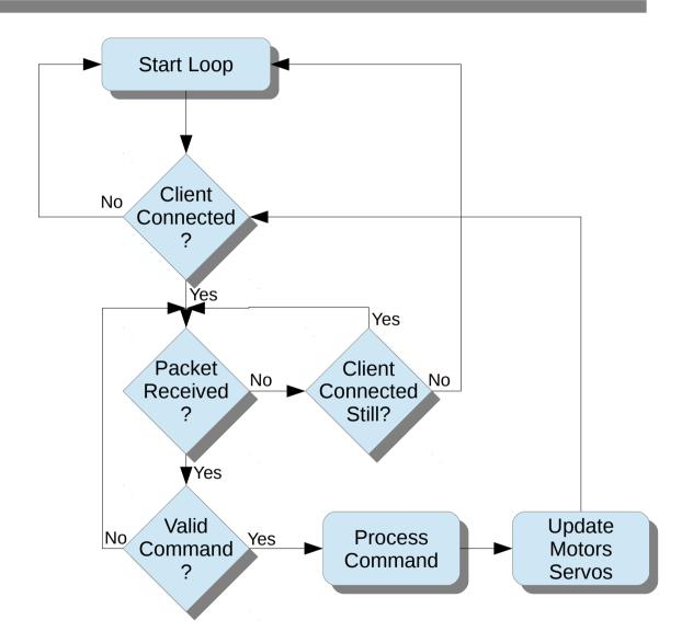
The flow chart helps show how the program operates. The diamonds are decisions the program makes using commands like if(). The rectangles are the actions taken such as adjusting the servo angles and the speed of the motors.
