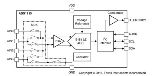
• The ADC module provides easy connections.
