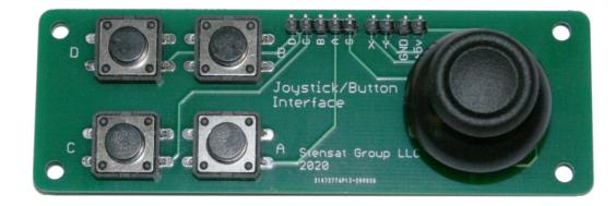
• The joystick module consists of four tactile push buttons and an analog joystick that includes a button activated by pressing the joystick knob.
